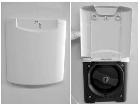
Fig. 20: Fresh water intake port
