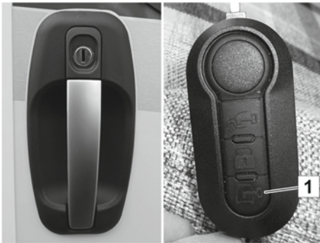
Fig. 10: Door handle, key with remote control for the central locking system
