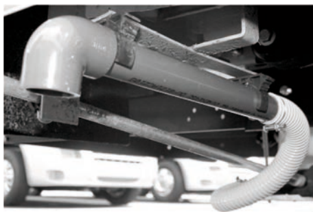
Fig. 84: Drainage outlet, example
