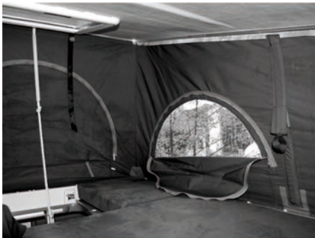
Fig. 37: Pop-up roof, interior
