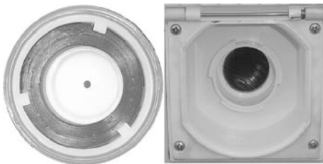
Fig. 79: Twist cap (left), fresh water intake port (right)
