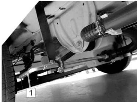
Fig. 83: Linkage assembly for drain valve, example
