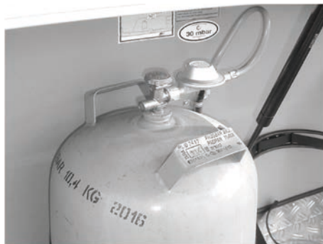
Fig. 68: Gas bottle with low pressure regulator and low pressure hose
