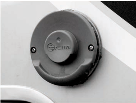
Fig. 74: Wall exhaust stack
