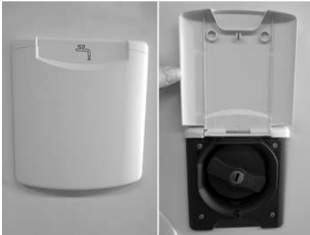
Fig. 78: Fresh water intake port
