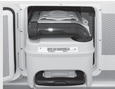
Fig. 49: Waste holding tank
