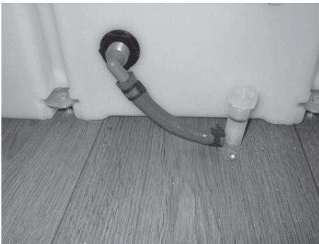
Fig. 97: Drain valve, example
