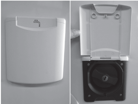
Fig. 106: Fresh water intake port
