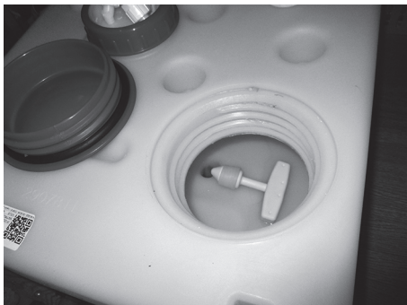
Fig. 99: Drain plug in the fresh water tank
