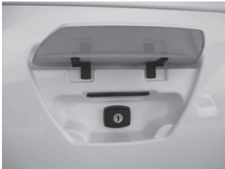
Fig. 75: Gas locker lock
