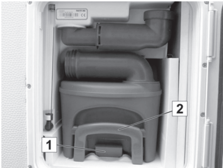
Fig. 199: Waste holding tank in the disposal shaft
