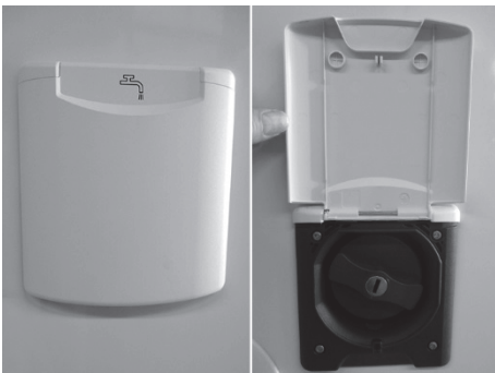
Fig. 23: Fresh water intake port
