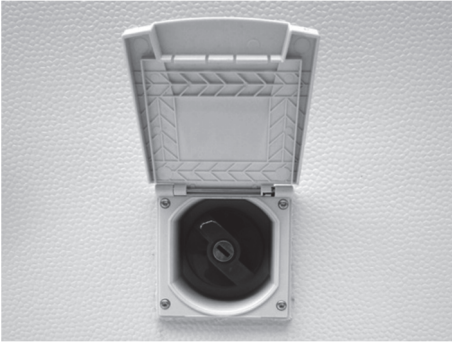
Fig. 95: Fresh water intake port
