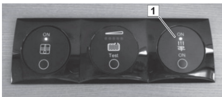
Fig. 94: On-Off switch of the floor heating system
